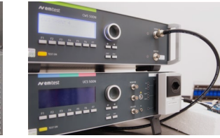
Generators for Surge and Burst
