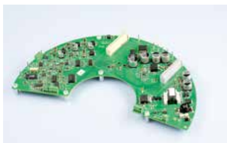
Multispectral LED based photometer module with lock-in amplifier
