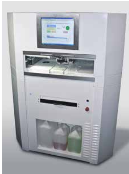
Automated extraction of multiple frozen aliquots from a single frozen biological sample
