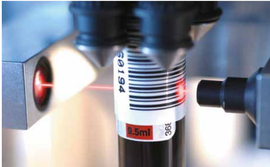
Laser based tube inspection unit for clinical diagnostics
