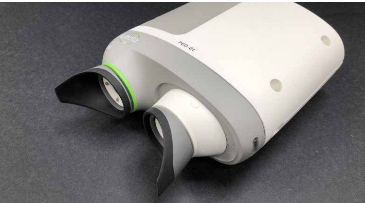
The retinal health monitor keeps track of the progression of retinal diseases by means of optical coherence tomography. The patient uses the device regularly at home, and the data recorded are automatically processed and transferred so that treatment can be monitored.
