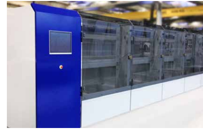
Automated, integrated production line for solar panels
