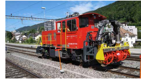
Retrofit of a Swiss Federal Railways small snow blower into a special railway vehicle
