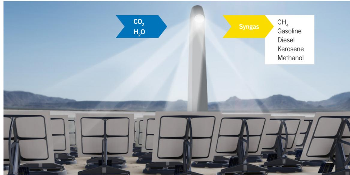
System with solar tower, heliostats and receiver in focus
