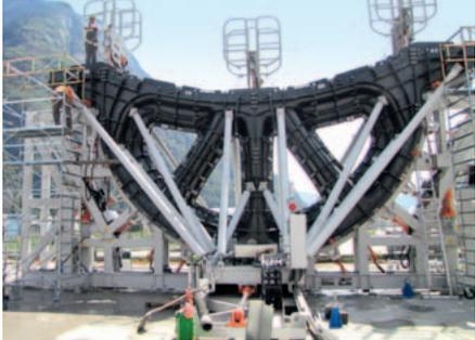
**Concrete casting machine for the support structures of CSP solar systems**
