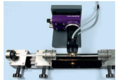
Optical in-line quality check in the production of an implant
